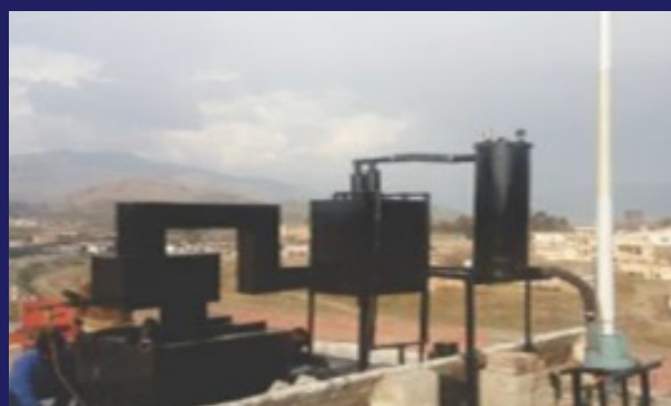
Incinerator and pollution control device at Azam Memorial Hospital Havellian
